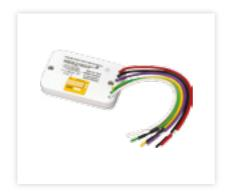
The XP95A Isolator is placed at intervals on the loop and ensures that, in the case of a short-circuit, only the section between the isolators will be affected. When the short-circuit is removed, the isolators automatically restore power and data to the isolated section.
