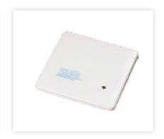
The XP95A Mini Priority Switch Monitor Module is designed to monitor the state of one or more single pole, voltage-free contacts and to report the status to Apollo compatible analogue control equipment. It can also place a signal on the loop to provide early warning if a device such as a pull station is operated.
