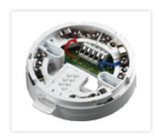
All detectors in the Discovery range fit the Intelligent Mounting Base. The mounting base is a low insertion force base with stainless steel contacts for the detector terminals. XPERT cards are supplied with all bases.
