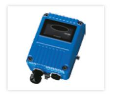
The IS IR<sup>3</sup> Flame Detector is designed for harsh environments in either indoor or outdoor applications. It is sensitive to low-frequency flickering IR radiation emitted from flames during combustion. The sensor operates even through a layer of oil, dust, water vapour or ice. These detectors have been approved by Baseefa to EN50014, EN50020 and EN50284. The requirements of Directive 94/9/EC, the Atmosphere Explosives ATEX Directive have also been met.
