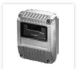
The Intelligent IR<sup>2</sup> Flame Detector is designed for harsh environments in indoor applications. The detector has two sensors which respond to different IR wavelengths to discriminate between flames and spurious sources of radiation.
