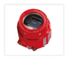
The Flameproof UV/IR<sup>2</sup> Flame Detector is designed for hazardous environments in either indoor or outdoor applications where open fires may be expected. False alarms from flickering sunlight, arc welding or lightning are avoided by the combination of UV and dual IR signal processing techniques. It detects almost all flames, including those invisible to the naked eye, e.g. hydrogen fires. Certified by ISSOP for compliance with standards EN50014, EN50018 and EN50281.
