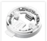
The Isolator is placed at intervals on the loop and ensures that, in the case of a short-circuit, only the section between the isolators will be affected. When the short-circuit is removed, the isolators automatically restore power and data to the isolated section.
